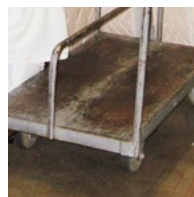
Metal—dents and rusts
