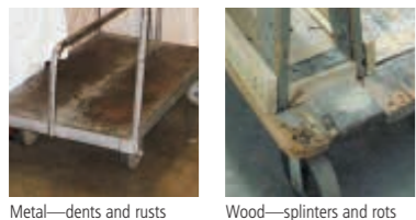
Metal—dents and rusts Wood—splinters and rots
